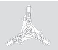
Determination of height of locator posts:  $\Delta$  = Distance between clamping position and locating face Height of locator posts [H] = 32,5 mm -  $\Delta$
