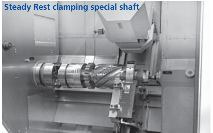
Steady Rest with diamond pads clamping input shaft in hard turning/grinding operation
