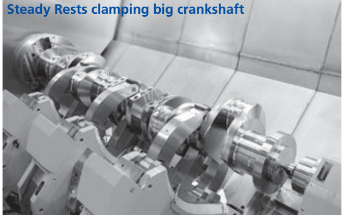
Steady Rest clamping special shaft
