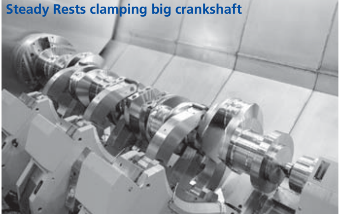
Steady Rest clamping special shaft
