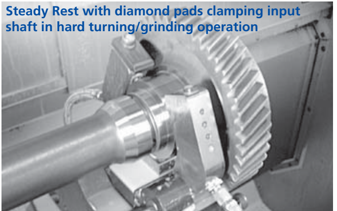
Steady Rest clamping aircraft shaft
